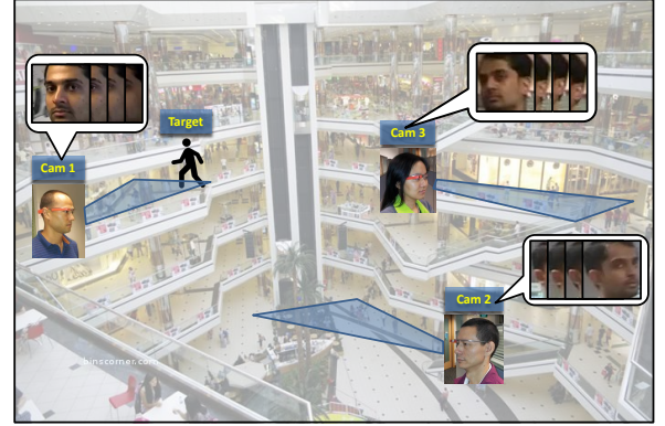
Fig. 1. Illustrative diagram for person re-identification using multiple first-person-view cameras. Three wearable devices (Google Glasses), shown as Cam 1-3, are worn by security personnels at different levels in a multi-stored congested shopping mall. As a target appears in the Field-of-View (FoV) of a camera (shown using trapezoidal regions on the ground plane), uncluttered face shots of the target can be observed and processed for re-identification.
